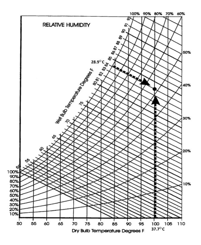
First find the dry temperature on the bottom of the chart, then find the wet bulb reading on the right hand curved line, follow the grid lines until the two intersect, and read off the humidity from the curved lines.
