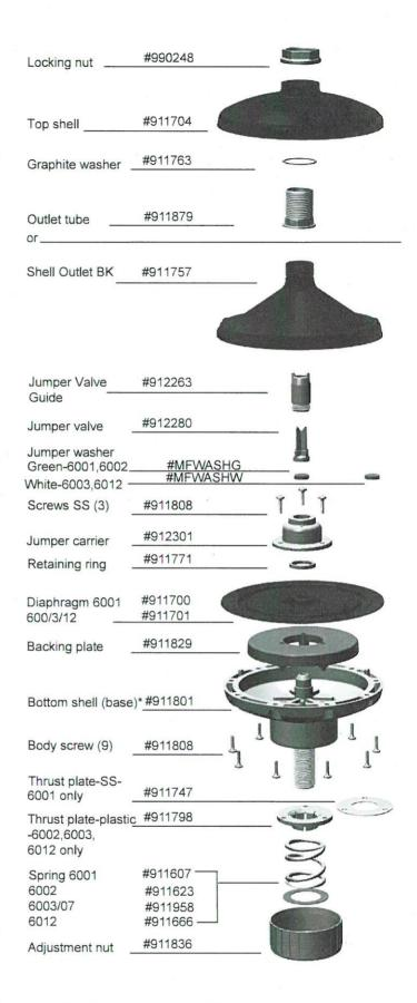
N.B Diaphragm bottom shell (base) and spring differ from model to model
