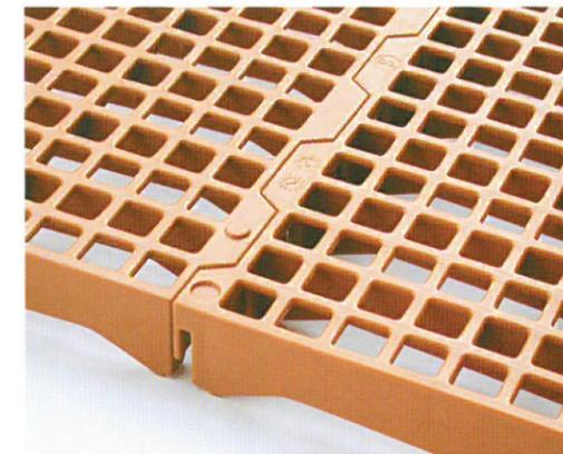
Aries and Orion SKA slats are made of pure polypropylene, very easy to clean and resistant to wear, to the differences in temperature and chemical agents. They have a self-supporting structure which only needs narrow steel bearers at 90 cm, protected and kept clean by the interlocking slat connections. Easy and quick assemble and dismantle.
