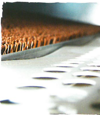
fondo nido e nastro raccolta uova nest bottom and perforated belt for collecting eggs
